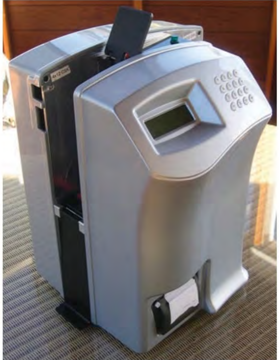
Design SMART has developed an enclosure for the electronic components of the Senztrak unit, a product which sits in trays of kiwifruit and detects any spoiling fruit.
