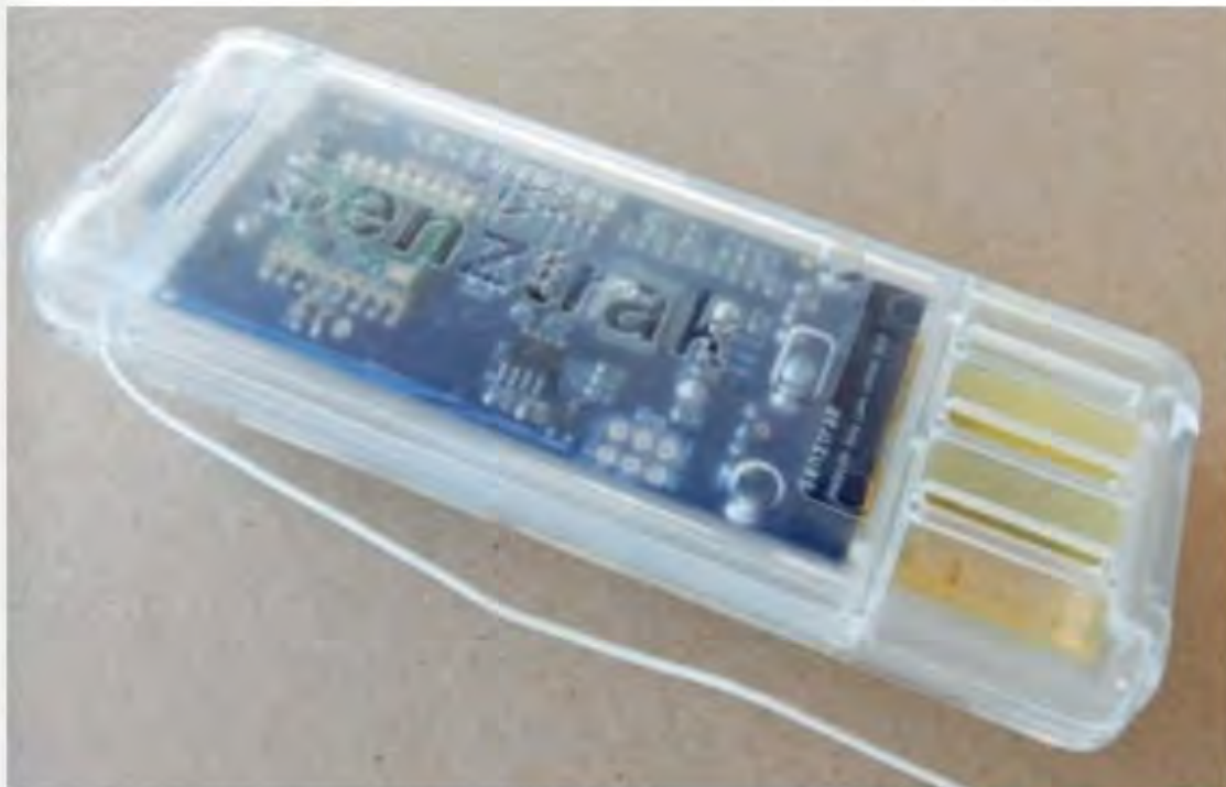
Design SMART has developed an enclosure for the electronic components of the Senztrak unit, a product which sits in trays of kiwifruit and detects any spoiling fruit.
